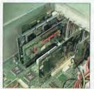
sound board on its Intel Aladdin series motherboard. A CrystaLake Wavetable upgrade card was included with the system. It adds complete General MIDI and Roland General Synthesizer compatibility to the Sound Blaster Pro and Microsoft Sound System digital capabilities integrated onto the motherboard.
